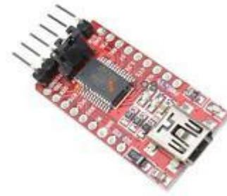
Connect a FTDI 232 USB serial adapter as shown above on the right to A9 and A10 pins on the STM32F103. Power the STM32F103 from either the FTDI module or from a USB cable connected between a PC and the STM32F103 USB connector. **Note if using the FTDI to power the STM32F103 ensure the correct voltage (jumper on FTDI) is selected and connected to the correct pin on the STM32F103.**
