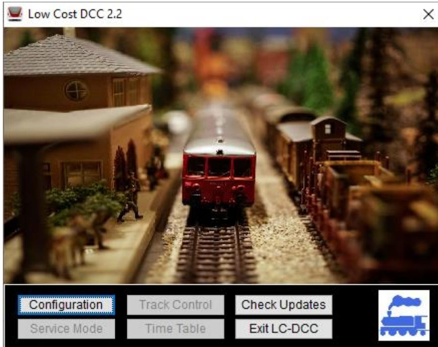
This screen provides the user with buttons to configure the DCC control system, check for software updates on the internet, exit the application and run the different operating modes of the DCC control software.
