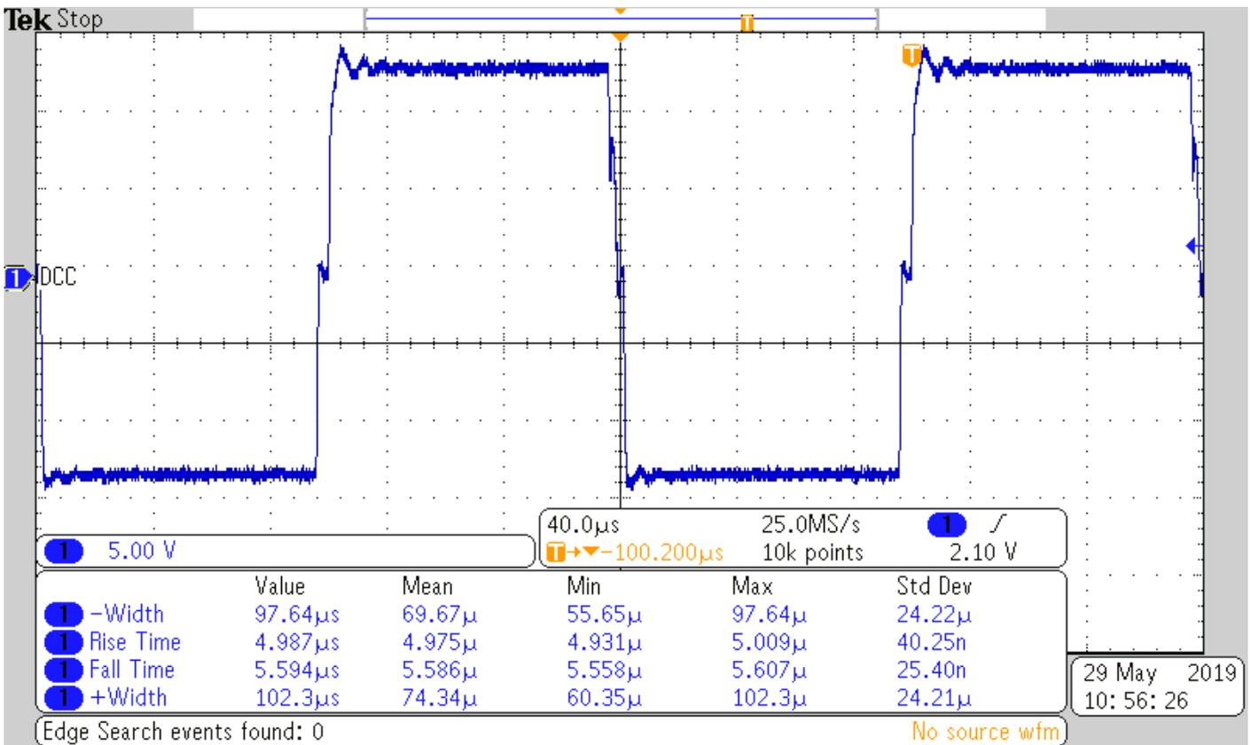
L298N Output 15V supply, 15 Ohm load
