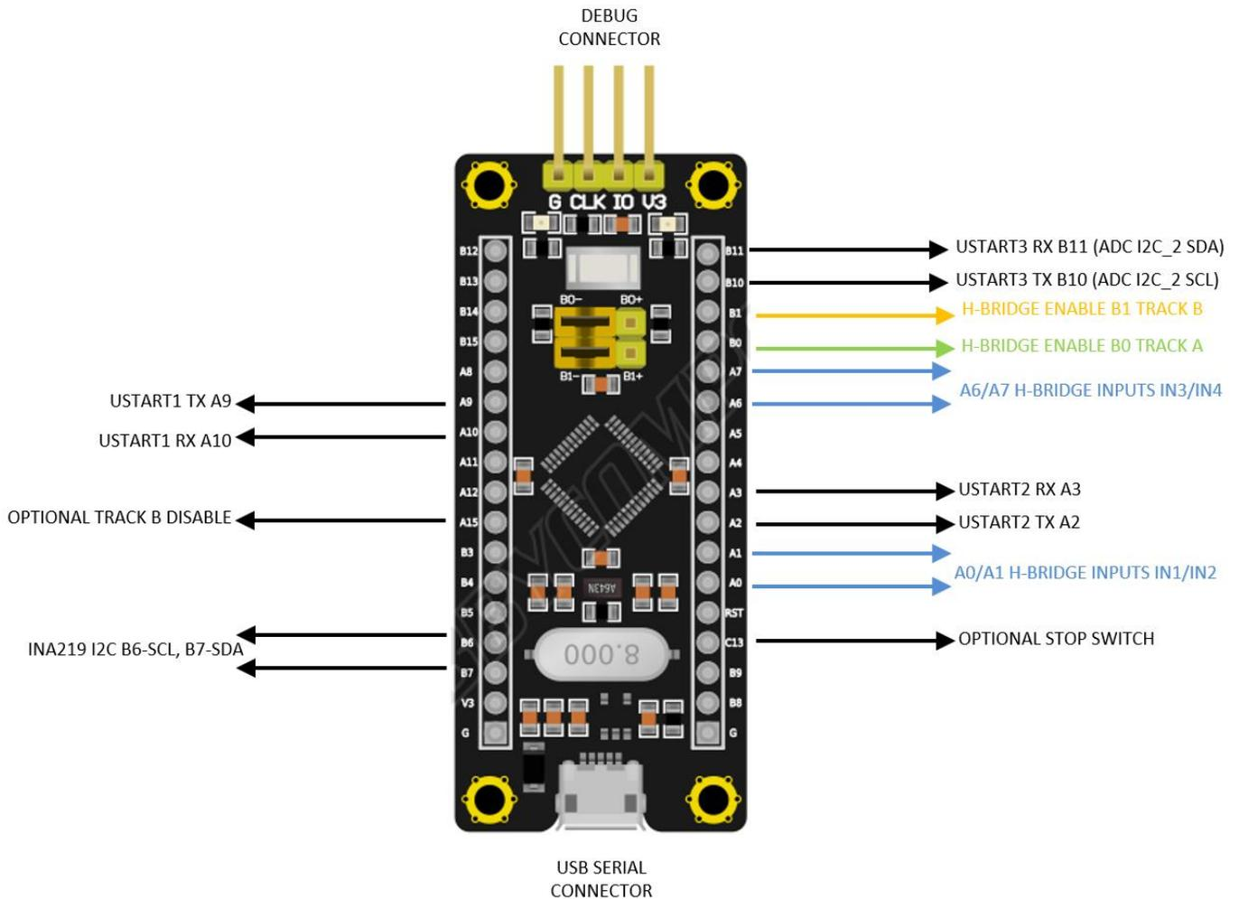
The USB connector is configured as a virtual communications port (VCP) so can be controlled using a Windows PC application. The USART connection can be connected to either an HC05 blue-tooth module or an FTDI USB serial adapter. Programming can be achieved by using a ST-LINK V2 USB programmer or by using USART1 and changing the boot jumpers (yellow in the above diagram).
