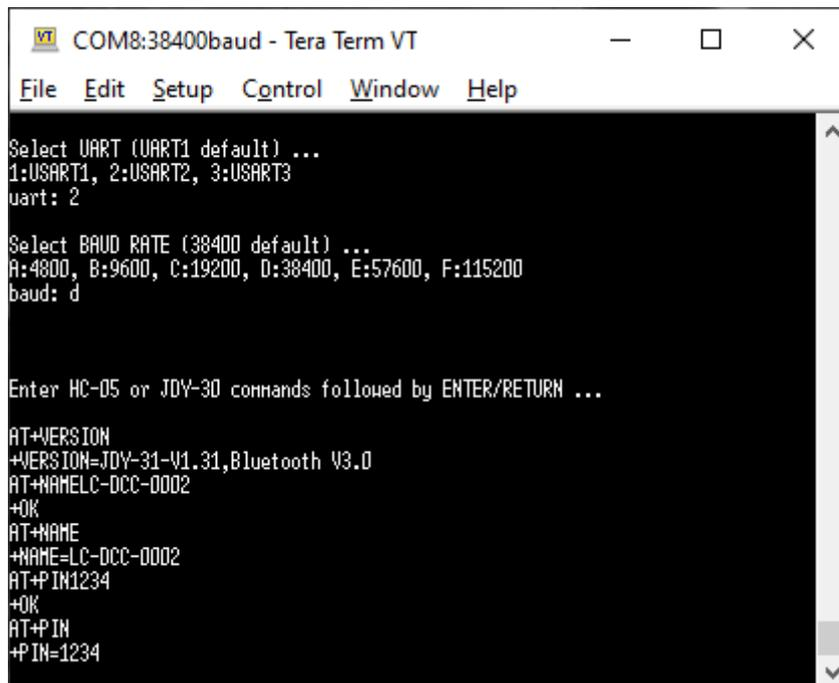
Note the JDY 30/31 is always in **AT command mode** until the blue-tooth is connected. To set the JDY 31 baud rate you must use the command **AT+BAUD6** for 38400 baud.
