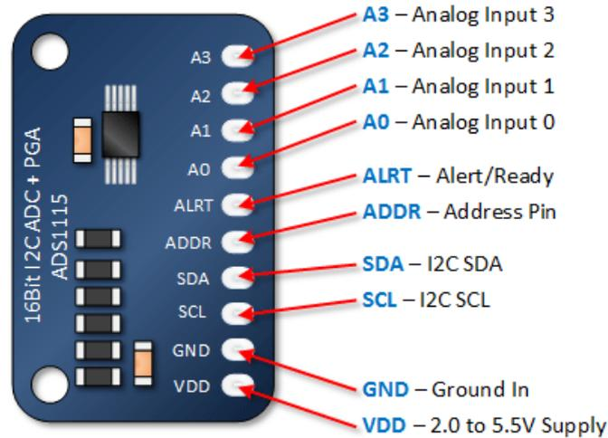
The ADDR pin must be connected to GND for the first ADS1115 and to VDD if a second ADS1115 is added. If two ADS1115 modules are used then the SDA and SCL lines from both modules need to be connected to the M3 or M4 processor.
