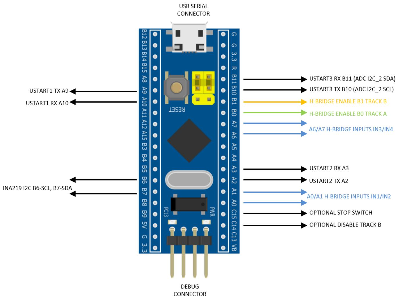
The USB connector is configured as a virtual communications port (VCP) so can be controlled using a Windows PC application. The USART connections can be connected to either HC05 blue-tooth modules or an FTDI USB serial adapters. Programming can be achieved by using a ST-LINK V2 USB programmer or by using USART1 and changing the boot jumpers (yellow in the above diagram).
