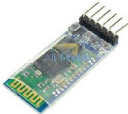
The blue tooth module must be configured to operate at 38400 baud. This can be done by using the blue tooth terminal application for the M3 or M4 processor found in the downloadable file `bt_terminal.zip`.
