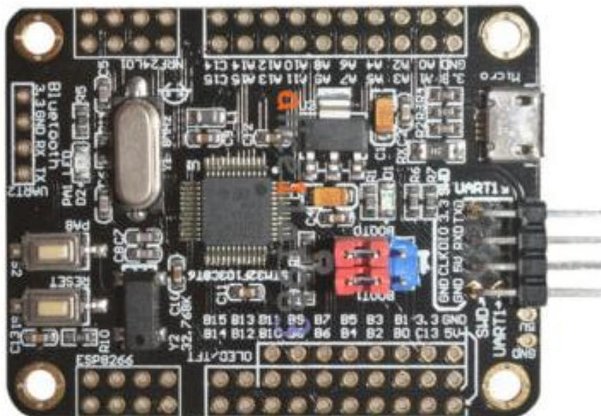
The ESP8266 module is mounted on the connector labelled ESP266 (bottom left in image above). The following connections are required to the H-Bridge and INA219 if connected.
