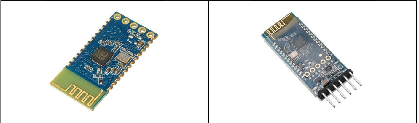
The blue tooth module must be configured to operate at 38400 baud. This can be done by using the blue tooth terminal application for the M3 or M4 processor found in the downloadable file `bt_terminal.zip`.
